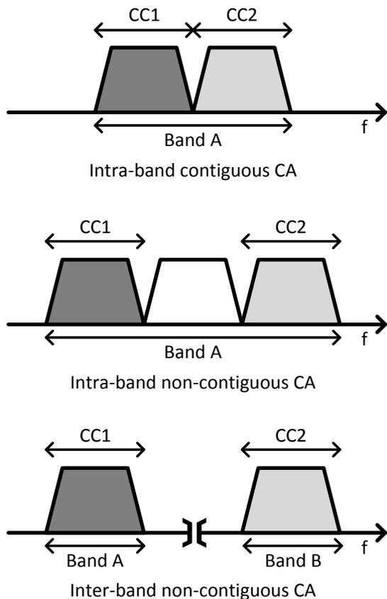
Fig. 1. The specified CA scenarios for LTE-Advanced.
